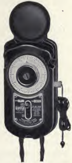
FIG. 54.—Automatic treatment timer and patient's release. (Courtesy of the General Electric X-ray Corporation.)
